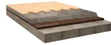
Slab and Floors Support for nailed flooring
