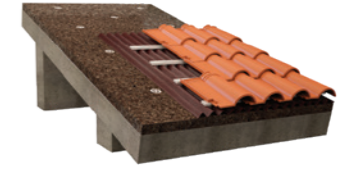
Roofs Pitched roof with corrugated roofing system
