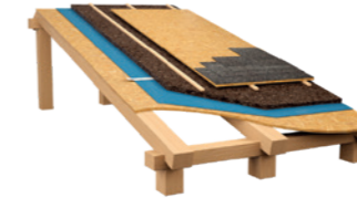
Roofs Pitched roof with above rafter insulation
