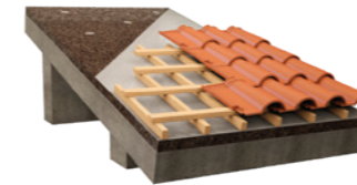
Roofs Pitched roof with roof membrane
