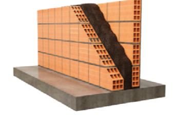
Internal partitions Filling the internal double walls with expanded cork granules
