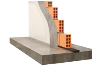
Internal partitions Masonry wall and slab discontinuity
