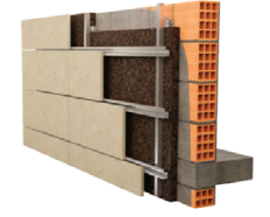
External walls Exterior cladding - cork at sight wave facade s1
